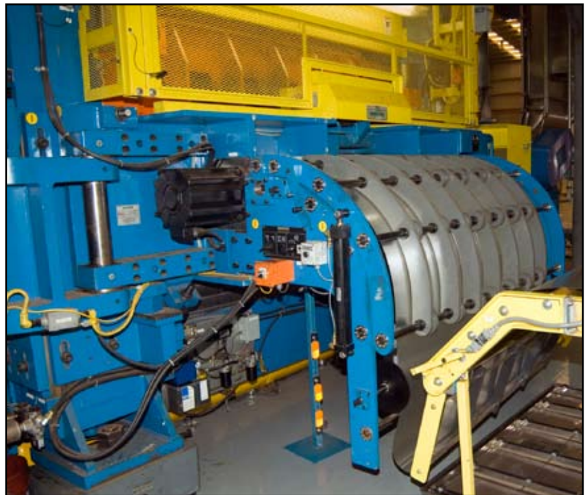
Minster's new MSCF-72 servo cupper feed has helped increase productivity at Modelo's Zacatecas Can Plant.
