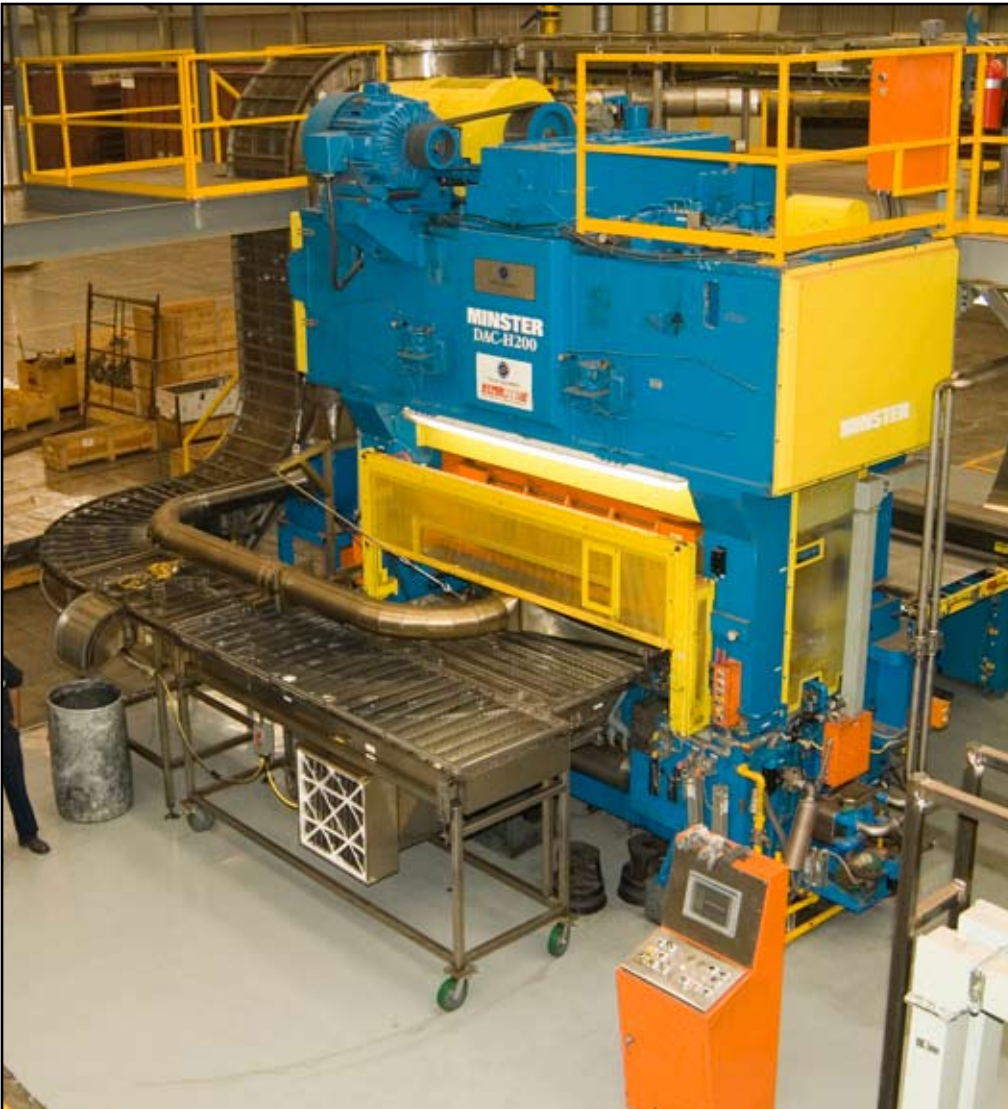
The Minster DAC-H200 press is an integral component of Stolle Machinery's Hyperdyne System, recognized as the highest production cupper system available in the can industry.
