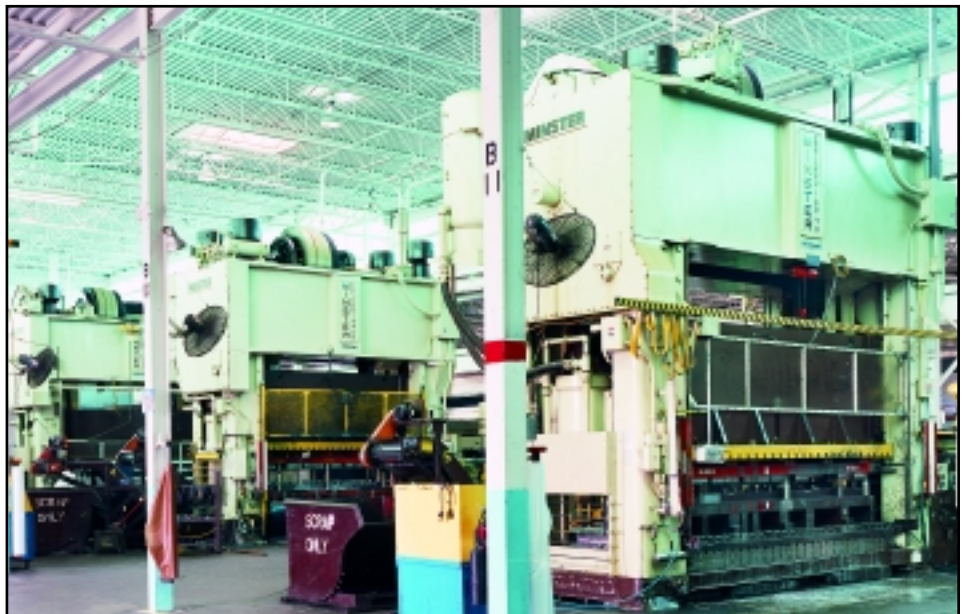
Three Minster E2-1000 ton presses perform some of the big jobs at Schaller.
