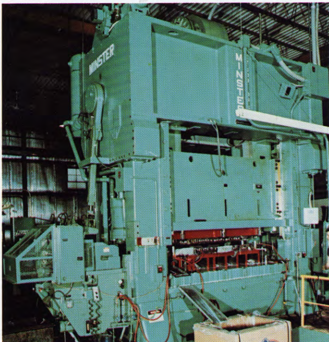
Regal Metal Products' newest Minster is an E2-600-108 featuring pendant-mounted operator's controls and a double-roll Minster Electronic Feed capable of handling material up to 32" wide.
