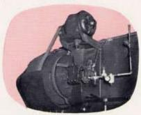
This Minster air-operated combination friction clutch and brake unit on #50-5 ½-72-2216 has operated 13 years. This clutch and the others on Minster Presses at New Idea have never been disassembled.
