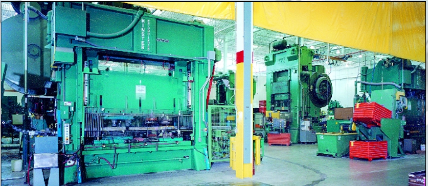
These two Minster E2 presses help perform secondary stamping operations.
