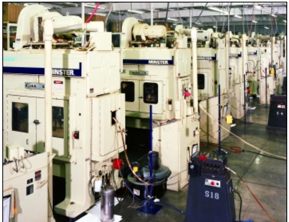
Numerous Minster Pulsar presses stamp out electrical connector parts at speeds of up to 1200 strokes per minute.
