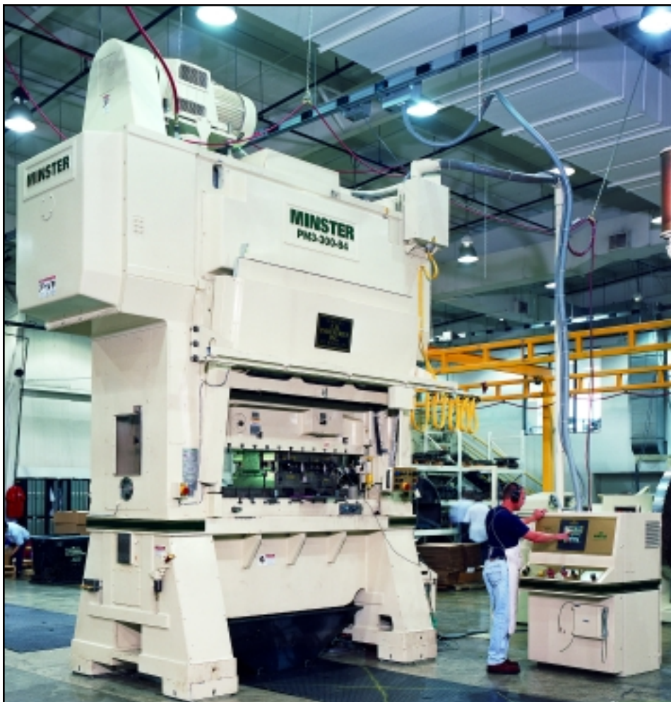
A Minster PM3-300 press was recently installed at L.H. Industries' lamination stamping facility.
