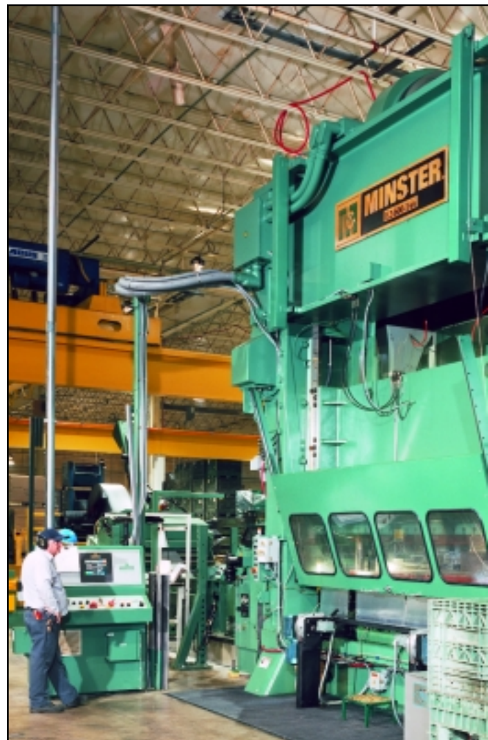
Hatch's newest Minster press -- this E2 600 -- includes the M integration with the Minster material handling line.
