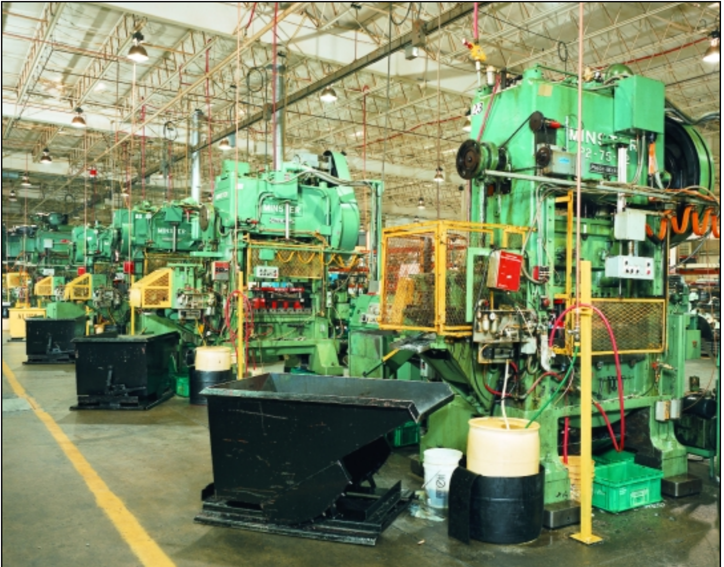
Several Minster P2 Piece Maker presses at the Hatch Stamping Company.
