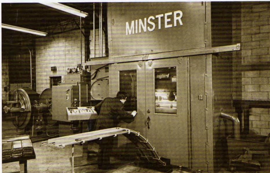
Hummingbird line includes Minster coiled material handling system, Minster Cam Feed, press within noise enclosure. (A box stripper in this die forms a tunnel into which scrap slugs drop and are then blown into the container outside the enclosure.)
