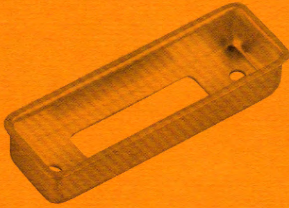
Pin and seal housing from .025" Aluminum in 4 operations with \pm 0.002 tolerance. Usually run in 5000 quantity on Die-Namic press.
