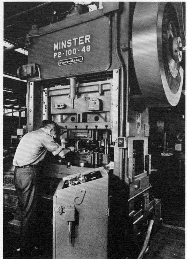
P2-100 automatic production press with Die-Namic fixture.
