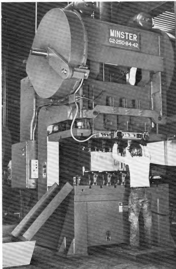
Minster G2-250 gap press is driven from both ends of the crankshaft to eliminate torsional deflection found in presses driven only from one end.
